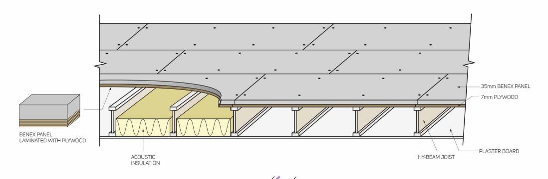
NOTE: • SCREWS 75mm CHIP BOARD TREATED PINE COATING
